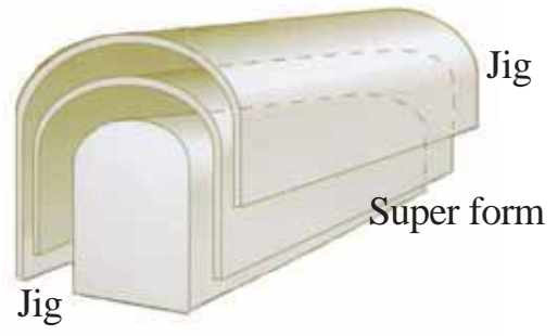
Fig : (b) Jig method veneering/covering in one process
