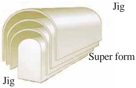
Fig : (a) Jig method for multiple shapes
